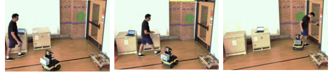
(d) DWA: Initial time step. (e) DWA: Robot does not yield to human. (f) DWA: Robot collides with human.
