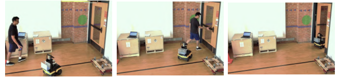
(a) Our approach: Initial time step. (b) Our approach: Robot yields to human. (c) Our approach: Robot follows through.
