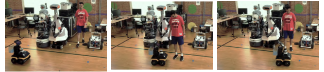
(j) DWA: Initial time step. (k) DWA: Robot stops when human slows. (l) DWA: Robot moves once human retreats.
