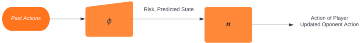
Fig. 4: The policy for Human and Robot Players side by side. \Phi and \zeta are neural networks which output risk, adaptation, and predicted oponent state and change in these values respectively.
