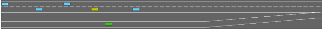
Fig. 1: Initial configuration of our highway merge environment. The yellow vehicle is the AV capable of sharing its intent. The green vehicle is the merging AV that receives the former’s intent. The blue vehicles are human-driven.
